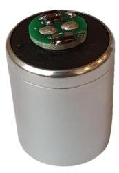
Based on the technology transfer for manufacturing the SM® range of geophones from Sensor® Nederland BV, HGS (India) Limited (erstwhile Geosource India Limited) offers the HG-6 LF geophone with 2 Hz natural frequency for picking up low frequency and deep level signals. The low frequency response is attained by the addition of a resistor - capacitor (RC) network.
